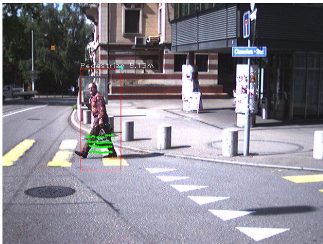
Fig. 6. Tracking a pedestrian that crosses the road. A bounding box surrounds the tracked object with annotated distance and a colored marker that refers to the track in the laser plane. In the laser plane it is visible a false track associated with one steady detection of a cylinder concrete by the laser based detector. For clarity, the laser tracked cluster is plotted into the image (green points).
