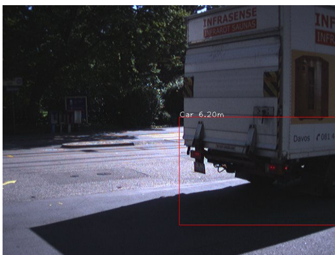
Fig. 7. Tracking cars in an intersection. A bounding box surrounds the tracked object with annotated distance and a colored marker that refers to the track in the laser plane. It is important to notice that also in case of the extreme closeup of the truck the track is still maintained
