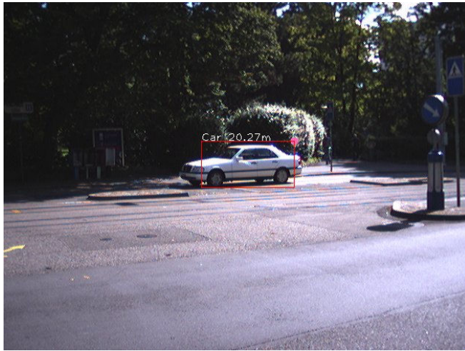
Fig. 5. Tracking cars in an intersection. A bounding box surrounds the tracked object with annotated distance and a colored marker that refers to the track in the laser plane.
