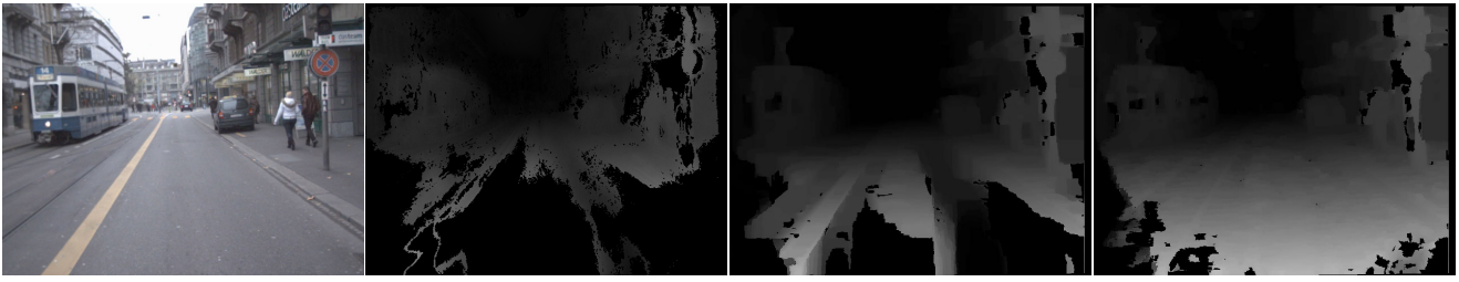
Fig. 5. Example stereo depth maps for a given image. From left to right: GPU-based [4] (20 ms), belief-propagation based [11] (20–30 s), global optimization [29] (30–40 s) algorithm. Parts that are believed to be inaccurate (by a left-right check) are painted black. More advanced algorithms give visually better results, but take more time and are often not necessary (see text).
