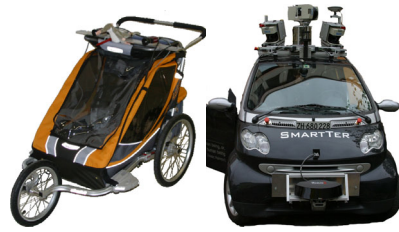
Fig. 2. Mobile recording platforms used in our experiments. Note that in this paper we only employ image information from a stereo camera pair and do not make use of other sensors such as GPS or LIDAR.
