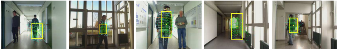
Fig. 4. Successful tracking. Green points: particles that matched to target; cyan points: particles that didn't match. Rectangles show estimated target state.
