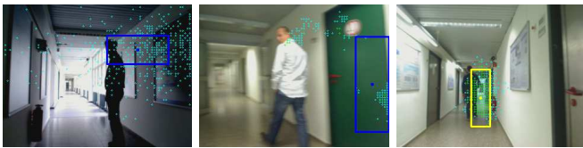
Fig. 5. Failed tracking. The points denote the particles (green points: particles that matched to the target, cyan points: particles that did not match). Rectangles denote the estimated target state (blue: less than 50% of particles match, otherwise yellow).
