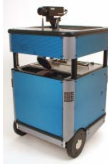
Figure 4: Pygmalion, the robot which was used in the experiments. It is a VME based system with a six axis robot controller. The processor board carries currently a PowerPC at 100MHz. Besides wheel encoders and bumpers, the sensory system includes the laser range finder and the CCD camera discussed in the second chapter.
