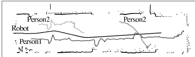
Fig. 6. Trajectories of robot and people in experiment 4. Person 1 is constantly tracked, person 2 receives a new identifier when reentering the sensor's field of view.
