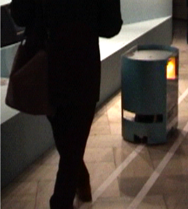
Figure 1. The “museomobil” at the opening of one of the exhibitions. The guide wires can be seen as white stripes. The conductive part of the guide was realized using “copper tape”
