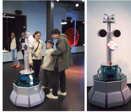
Figure 7. RoboX , the robot built for Expo.02. It sports two SICK LMS 200, a PowerPC G3 at 380 MHz and a Pentium III at 700 MHz.
