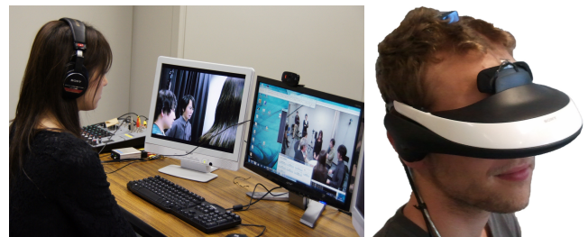
Fig. 2. The desktop-style tele-operation console currently in use for “Geminoid F” (left) and the head-mounted display (HMD, right), which will be used for tele-operation in this project
