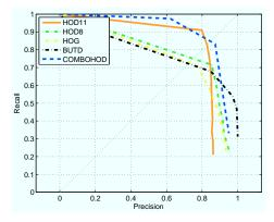
Fig. 3. Precision recall curves for depth-based, image-based, and combined RGB-D based detection methods. The most performant detector is Combo-HOD that combines both sensory cues. HOD is evaluated at different depth discretizations, 8bits and 11bits. HOD11 is the best depth-based detection method. Visual-based HOG detector underperforms due to unfavorable light conditions. BUTD underperforms due to the hyperbolic depth resolution loss of kinect data.
