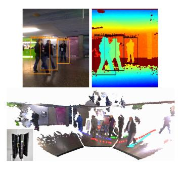
Fig. 1. **Top:** People detected in RGB-D data: dense depth data and color image data are simultaneously used for detecting a group of people. Note that the method neither relies on background learning nor on a ground plane assumption. **Bottom:** People tracking in RGB-D data by using a triple Kinect setup. The colored circles and dots in the point cloud show the positions and trajectories of five tracked persons.
