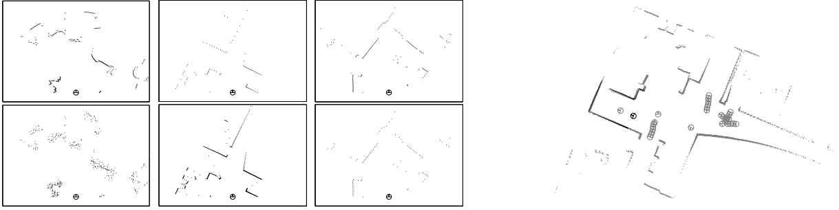
Fig. 4. Example locations and their transformations. Left, top row: reference locations, bottom row: same scans subject to extra Gaussian noise (bottom left, with \sigma = 0.25 ), oversampling (bottom center, 4 times), and subsampling (bottom right, 4 times). Right: View point changes given a reference location indicated by the black robot and the black laser points. The gray robots are map locations with a 50% overlap with the scan of the reference location.
